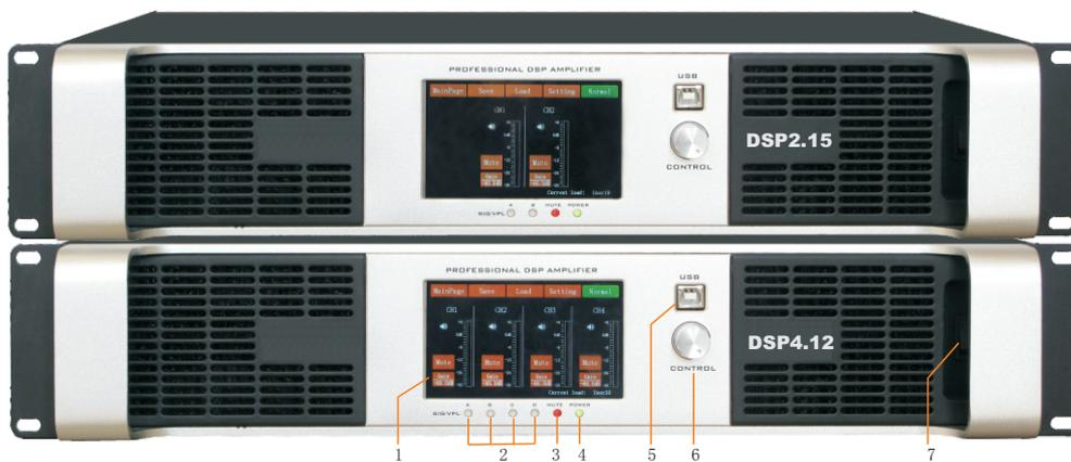
1-screen 2-signal/limiter (green is signal indicator, red is limiter indicator)
